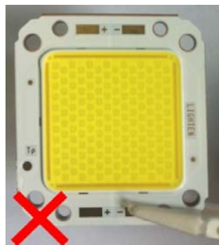
不可夾電極處 Don't clip both electrode
