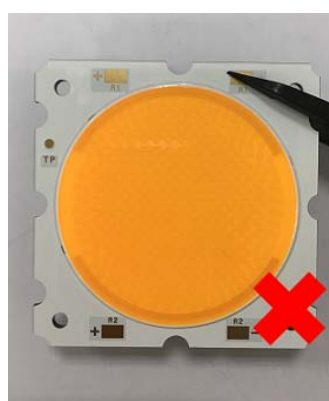
不可夾電極處 Don't clip both electrode
